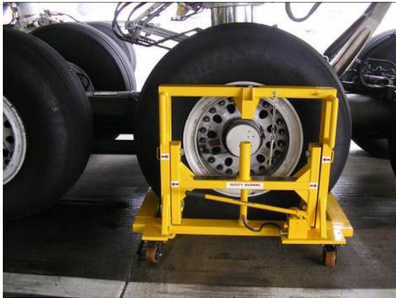
Aircraft maintenance engineers are frequently involved with the removal and replacement of aircraft wheels and brakes as part of regular maintenance and service requirements. Working in an industry where thousands of passengers each year rely on the maintenance staff to ensure aircraft are safety compliant, it is vital that engineers are provided with the appropriate ground support equipment to
