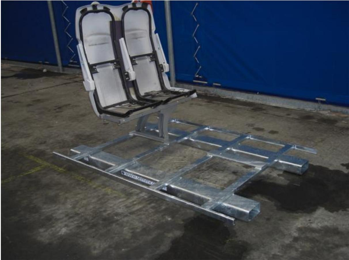
To enable and safely assist its workers with the essential refurbishment of its Class 222 Meridian Refreshment Project, East Midlands Trains employed Semmco Ltd to design and build purpose built staging and stillages. East Midlands Trains required manoeuvrable platforms that could transport the seats and carpets from the carriages as well as enable safe access for workers through the train double doors and carriages across the fleet.
