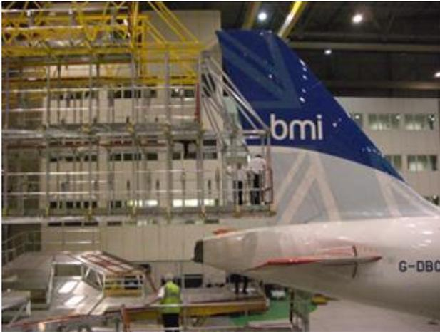
***Made to measure A320 tail docking system from Semmco proves instrumental in the implementation of bmi's equalised maintenance programme. This unique engineered solution has saved the cost of an entire plane over a 12-month period due to reduction in aircraft downtime. In addition the A320 tail dock has improved safety for aircraft engineering staff working at heights.***
