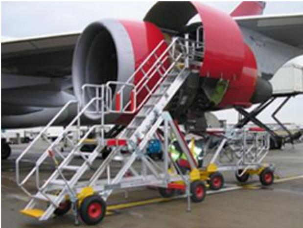
*Bespoke engine and cargo hold access solutions from Semmco improve safety for aircraft engineers whilst improving their productivity when working at heights.*
